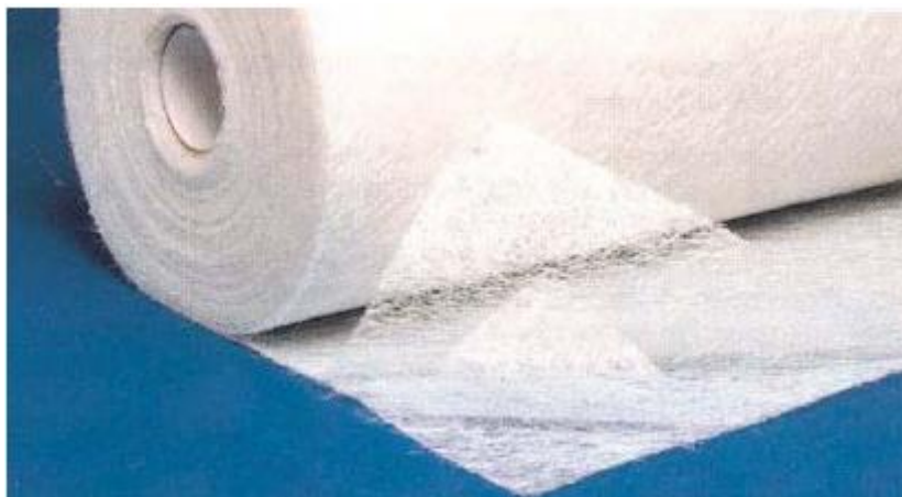
Figure 18 Typical glass fibre continuous filament mat (Chlosta 2012, p. 30)
