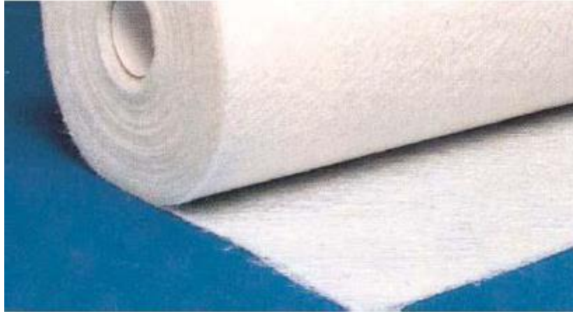
Figure 17 Typical glass fibre chopped strand mat (Chlosta 2012, p. 30)
