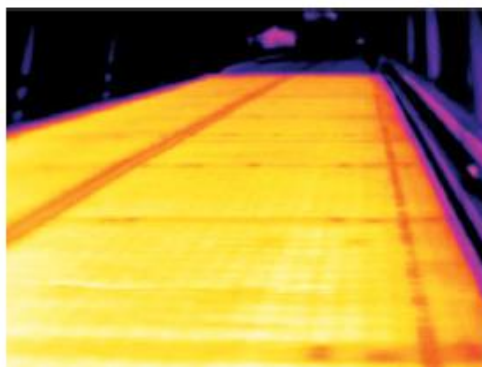
Figure 89 Thermography image of a bridge deck during heat source is applied (Meyer 2006)
