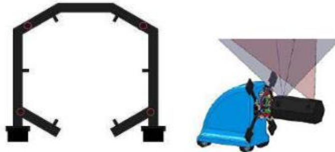
Figure 98 Left: C-Shape laser scan for external scanning; Right: Laser scanning system for internal inspection (UNIVPM et al. 2011)
