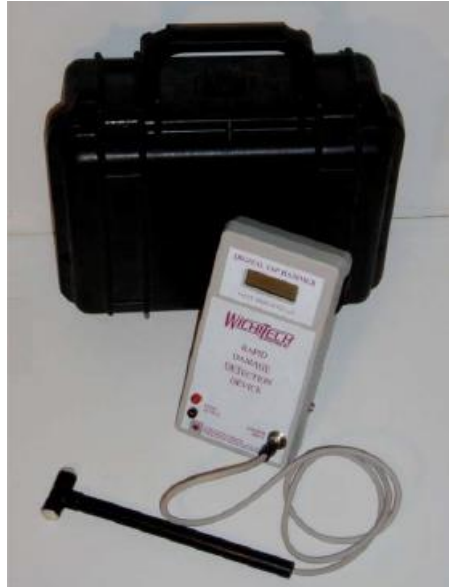
Figure 88 Electronic tap-test (Meyer 2006)
