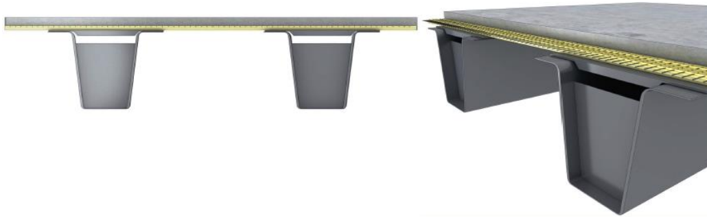
Figure 151 A section view and an overview of the position of a U-shaped beam (Warszawa 2009)
