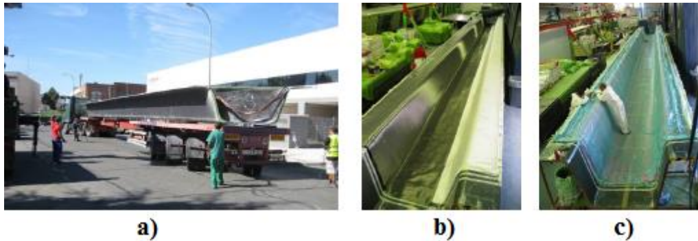
Figure 78 The Canary Island footbridge manufactured by the resin infused method a) Transportation of FRP girders b) and c) two phase manufacture of FRP girders (Hurtado et al. 2012, p. 5)
