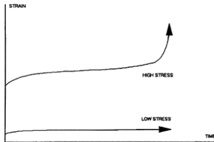
Figure 64 The creep behaviour of FRP composites subjected to high respective low loads (Clarke 1996, p. 253)
