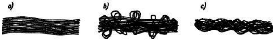
Figure 14 Various forms of rovings: a) smooth roving b) interlaced roving c) tangled roving (Potyrala 2011, p. 7)
