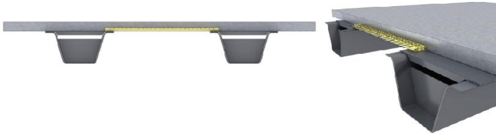
Figure 149 A section view of the deck position on open-shaped beam and an overview of the deck position on open-shaped beam (Warszawa 2009)
