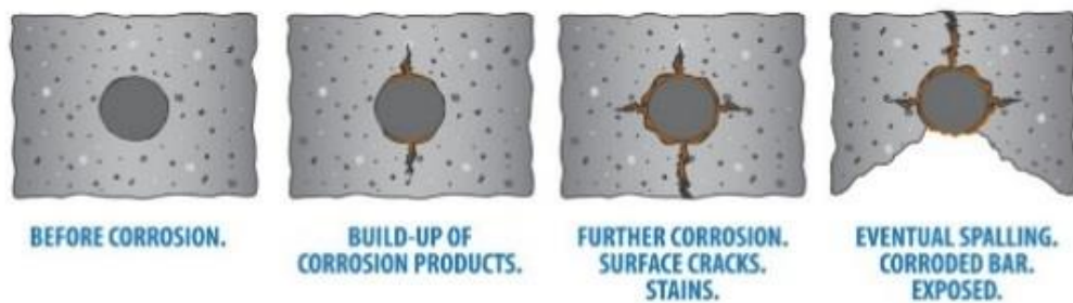
Figure 4 Cracking and spalling of the concrete due to internal reinforcement corrosion
