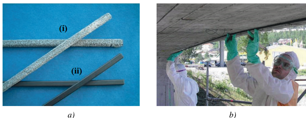
Figure 4.1 a) NSM-rods with (i) quartz sand compared to (ii) ordinary NSM-rods. b) Work performed using NSM-rods (Täljsten, Blanksvärd and Sas, 2016).
