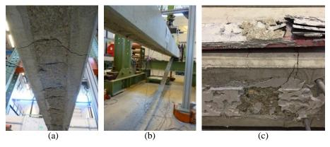
Figure 7. (a) Intermediate cracks; (b) Debonding of the laminate due to intermediate cracks in B2; (c) Rupture of the laminate in beam B3
