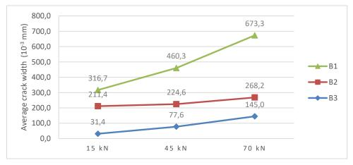
Figure 8. Average value of crack width in the 1.3-meter-long middle section (under constant bending moment) of beams at total vertical load of 15~kN, 45~kN and 70~kN
