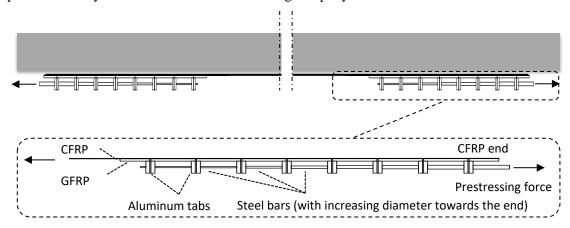
Figure 3. Applying prestressing force to CFRP laminate using the new technique
