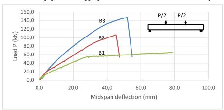
Figure 6. Load-deflection curves of beam specimens under four-point bending test
