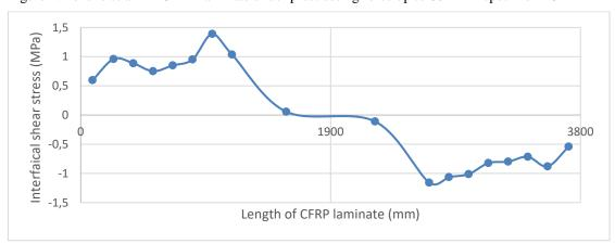
Figure 5. Interfacial shear stress between CFRP laminate and concrete beam under prestressing force of 80 kN in specimen B3
