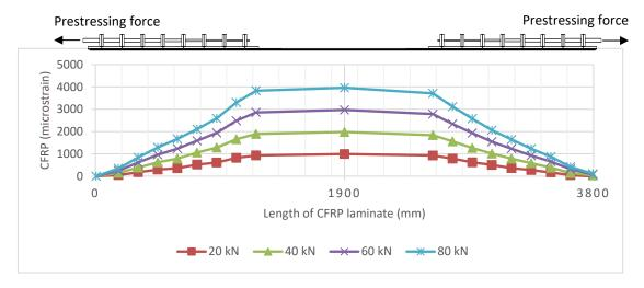
Figure 4. Tensile strain in CFRP laminate under prestressing force up to 80 kN in specimen B3
